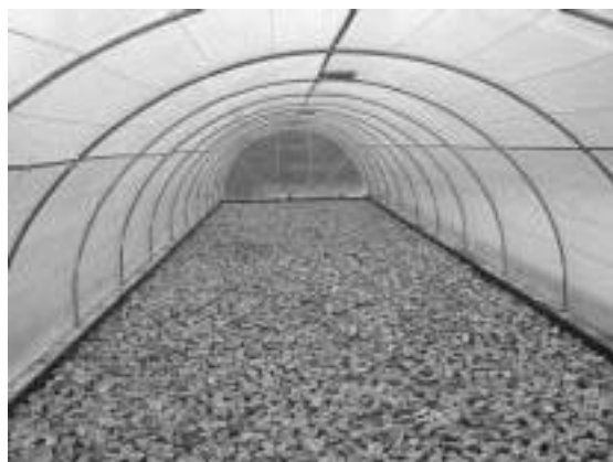
Fig.1. View of solar tunnel dryer with coconut kernels
