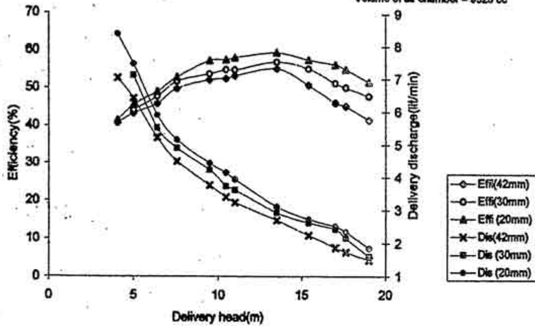
Fig.4 Effect of stroke length of waste valve on the performance of hydraulic ram
