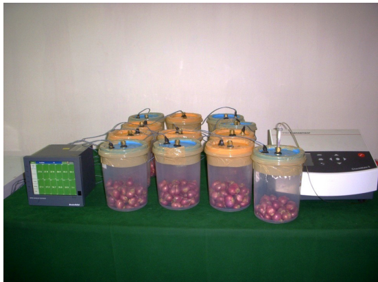
Fig. 1. Experimental setup for respiration rate measurement
