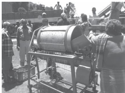
Fig. 4. Continuous type root vegetable washer in operation
