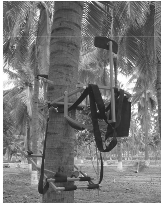
Fig.4. Ergo refined coconut tree climbing device fitted in tree
