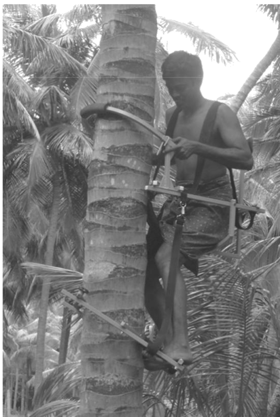
Fig.5. Operational view of ergo refined coconut tree climbing device
