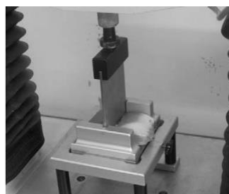
Fig.3. Cutting test of Aloe vera leaf sample
