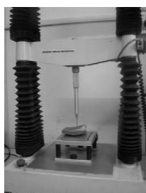
Fig. 2. Penetration test of Aloe vera leaf sample
