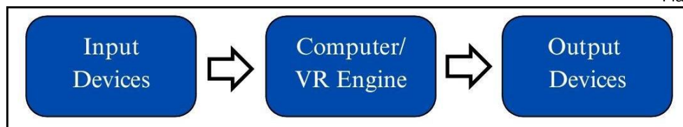
Figure 3: Basic data flow in a VR system from input devices through the VR engine to output devices
