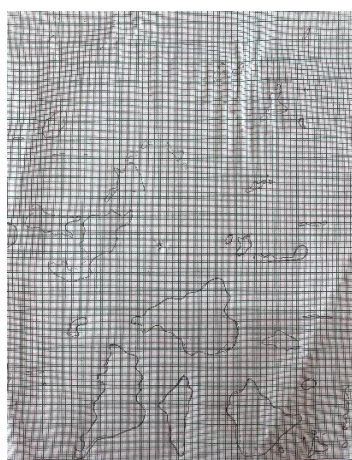
Figure 4. Graphical representation of corroded area
