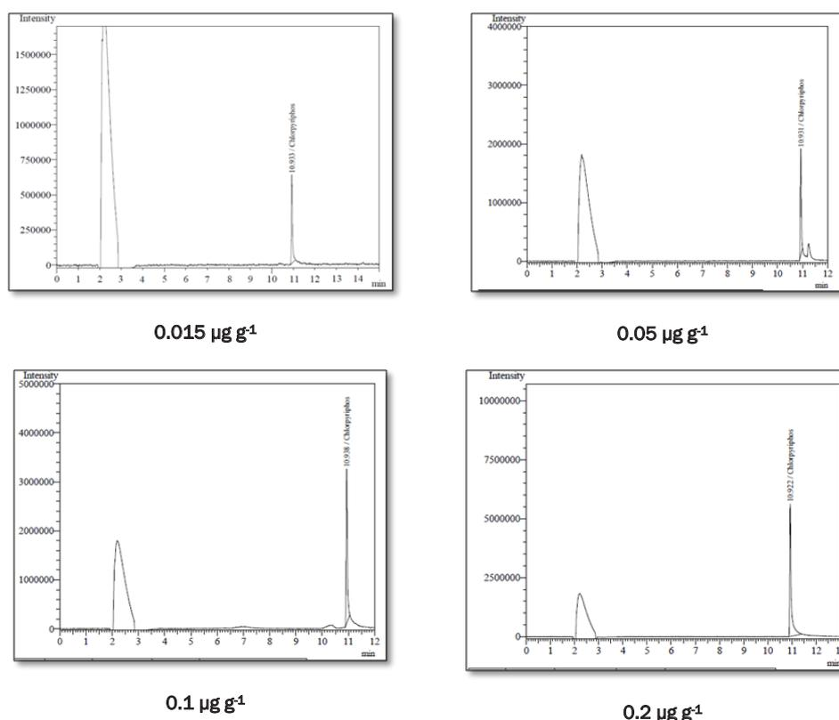
**Figure 1. Standard chromatograms of chlorpyrifos in Gas chromatograph**
