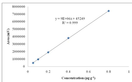
**Figure 2. Calibration curve of chlorpyrifos in gas chromatograph**
