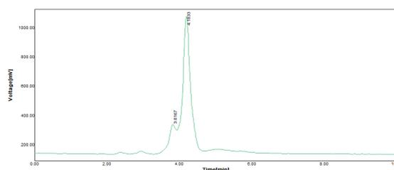
**Figure 6.** HPLC chromatogram of 24 h old culture grown in xylose and glycerol mixture. Peaks corresponding to xylose and xylitol were observed in 3.8 and 4.1 min. retention time respectively
