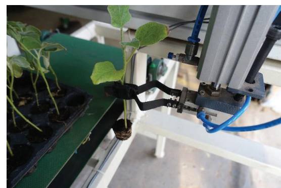
Fig. 3 Development of an experimental set up for an automatic transplanting mechanism
