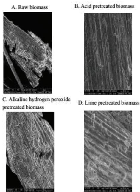
**Fig.1. SEM micrographs of pearl millet biomass**
