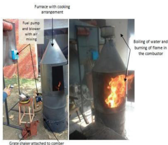
Fig.2.(a) Experimental set up for testing of bale combustor and (b) boiling performance test of bale combustor
